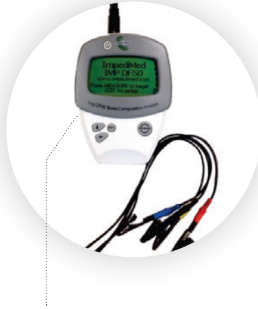
A device that measures body fat through bioimpedance may help to measure breast cancer risk.
